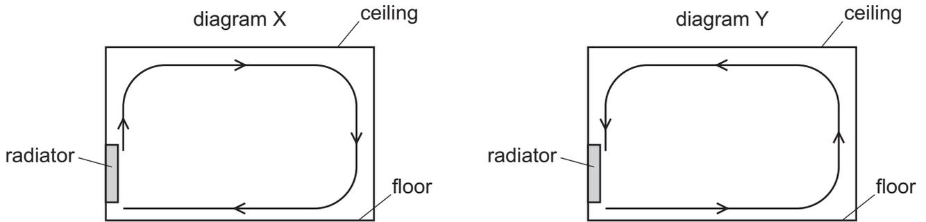
Which diagram and reason explain the heating of the room by convection?
