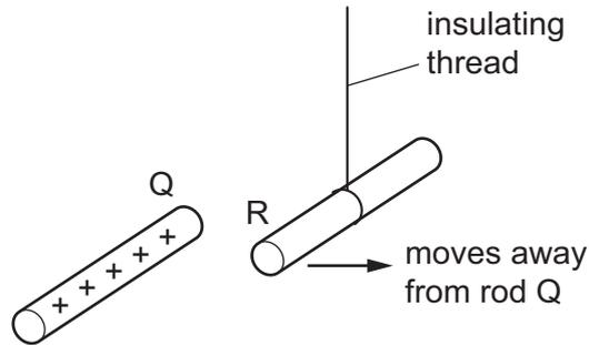
When the positively charged rod Q is brought close to rod R, rod R moves away from rod Q.
